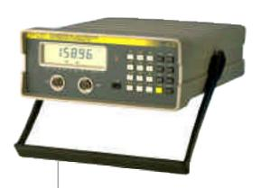
Thanks to its high performances and multiple functions, the PN 5207 is used as reference in quality department of various industries as well as in thermometry, physicochemistry, air conditioning or thermal exchanges laboratories, including calorimetry.
